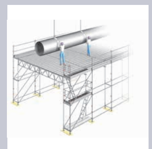
STAR with lattice beam as birdcage scaffolding
